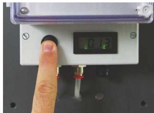
Measuring cell with mini LCD display for the local readings of chlorine residual and built-in temperature probe
